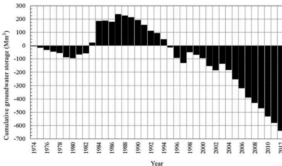
Figure 5. Cumulative aquifer storage volume between ‘Río Copiapó en La Puerta’ and ‘Río Copiapó en Angostura’ gauges. The reference (null) volume corresponds to 1973. Source: adapted from DGA (2013).
