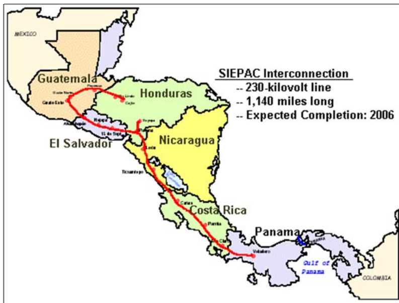
Figure 3.1: SIEPAC interconnection grid (Source: Guatemala Energy)
